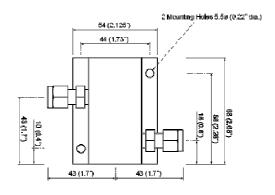
NOTE. The Assembly is shown with 1/4" OD tube fittings. The dimension across the tube fittings will vary for all other vive fittings.
